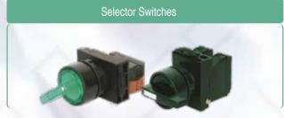
Illuminated /Non – Illuminated Various Voltage Rating AC.Dc24 V / 100-120V / 220-240 V /380 Normal / Long Shaft / key types 2/3 Position with spring return
